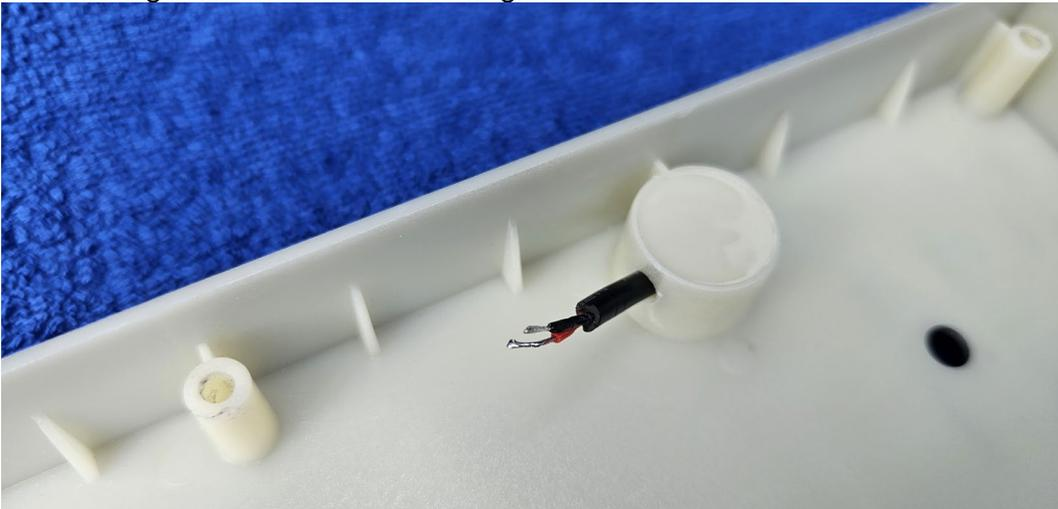
2. Connect the cable to the jack on the board. The two wires can be connected as desired (no polarity).
