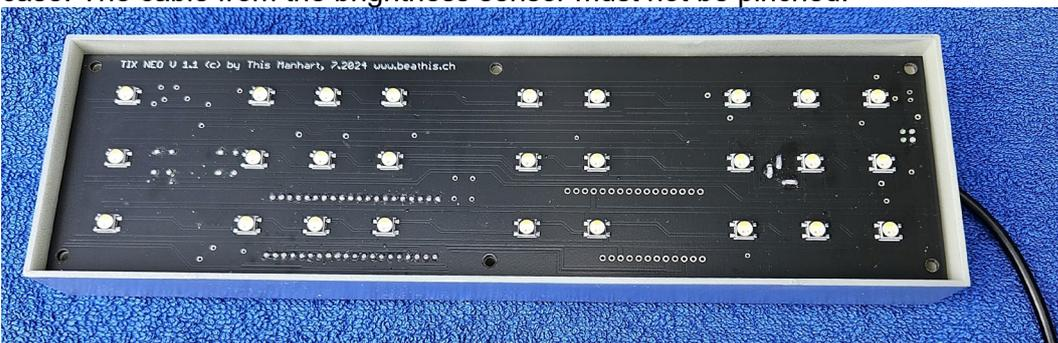
The buttons must not jam and a cracking sound must be audible when pressed.
