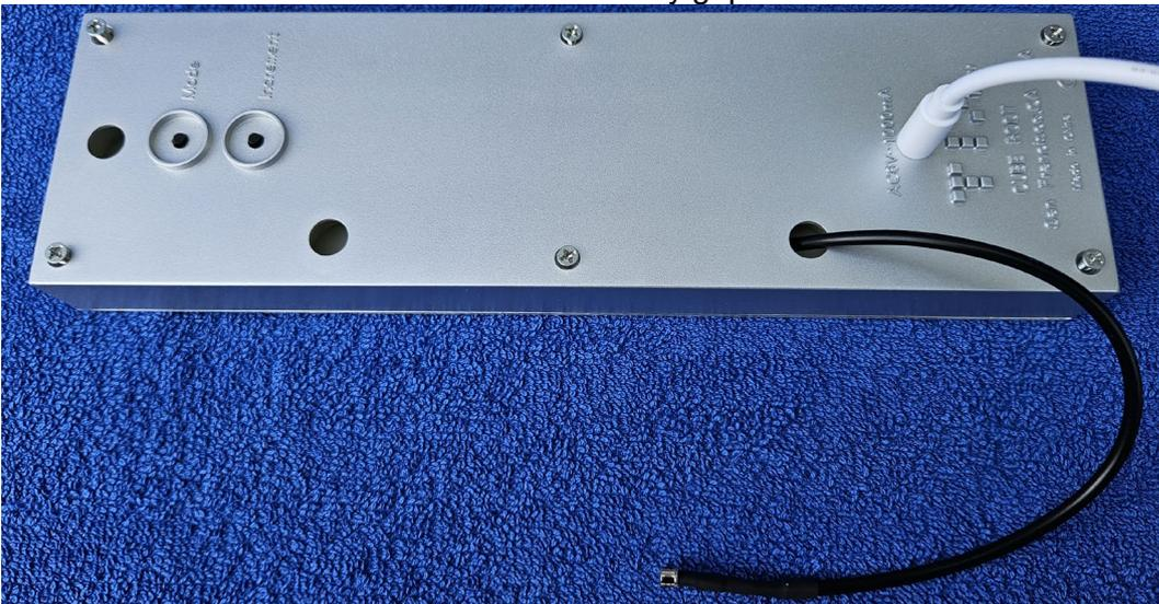
Note: The two buttons must have a clear pressure point when pressed (crack). If this is not the case, disassemble the TIX Clock again and enlarge holes for the buttons in the case with a fine file or a larger drill.
