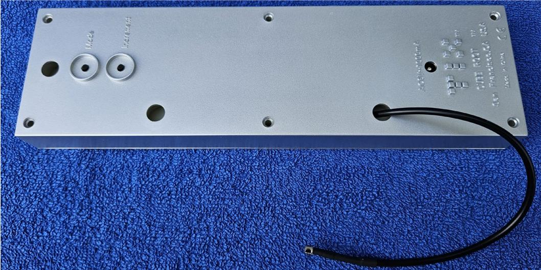
8. Plug in the new power cable and insert all 6 screws into the holes in the case. Screw in all the screws. Some of the screws do not immediately grip the thread.
