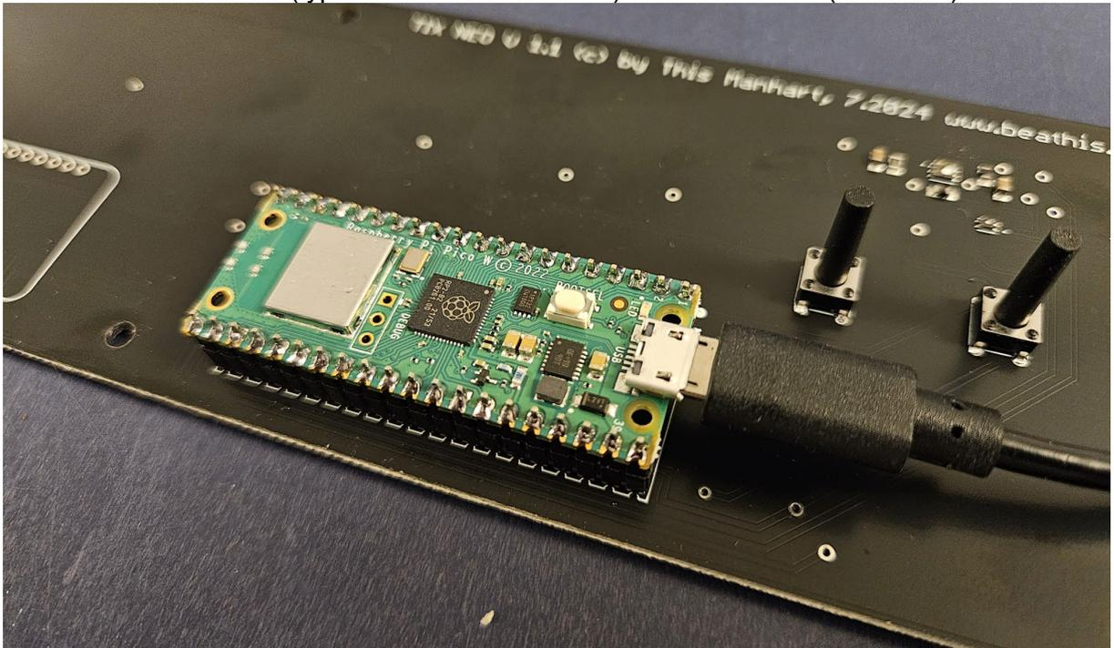
6. Press the button on the Pico 2 W module (arrow) and hold the button
