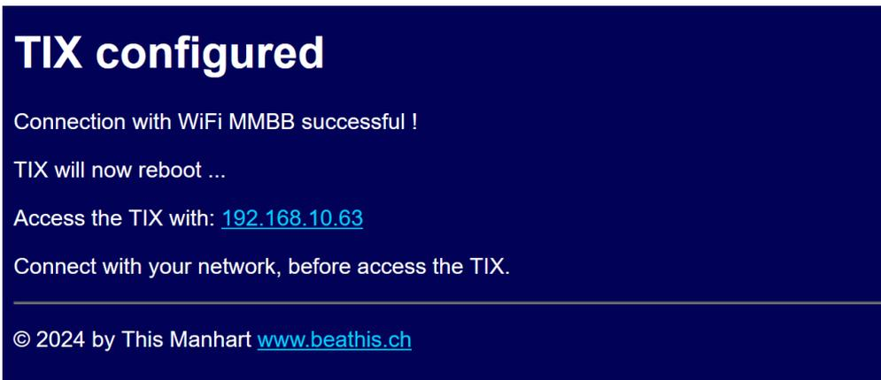
Connect the PC to the original Wi-Fi network and click the link with the IP address. The TIX Clock website opens.
