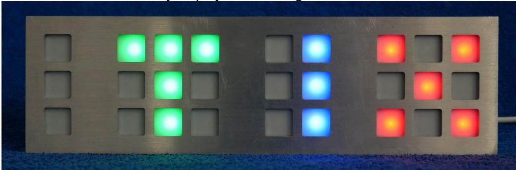
4. After a few seconds, the clock starts and shows a first time. The TIX clock starts at 01:00. The LED in the upper left corner flashes every second.
