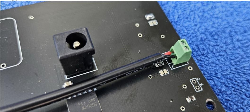
3. Carefully place the new board in the case. Make sure that the board is correctly aligned in the case. The cable from the brightness sensor must not be pinched.
